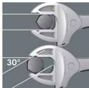
Thanks to the corner-width rectangular prisms, a back-pivoting angle of only 30° can be realized.
