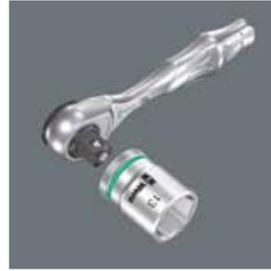
The Zyklop Mini 3 ratchet is the ideal tool for screwdriving in confined spaces. The fine tothing (60 teeth) allows a very low return angle of only 6°; the knurled wheel allows fast screwdriving even when there is no room for pivoting movement.
