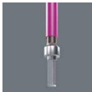
The clamping of the screw is achieved by a flexible locking ball. The holding function is especially helpful in confined, hard-to-reach spaces, where there is no room for a second hand to secure.
